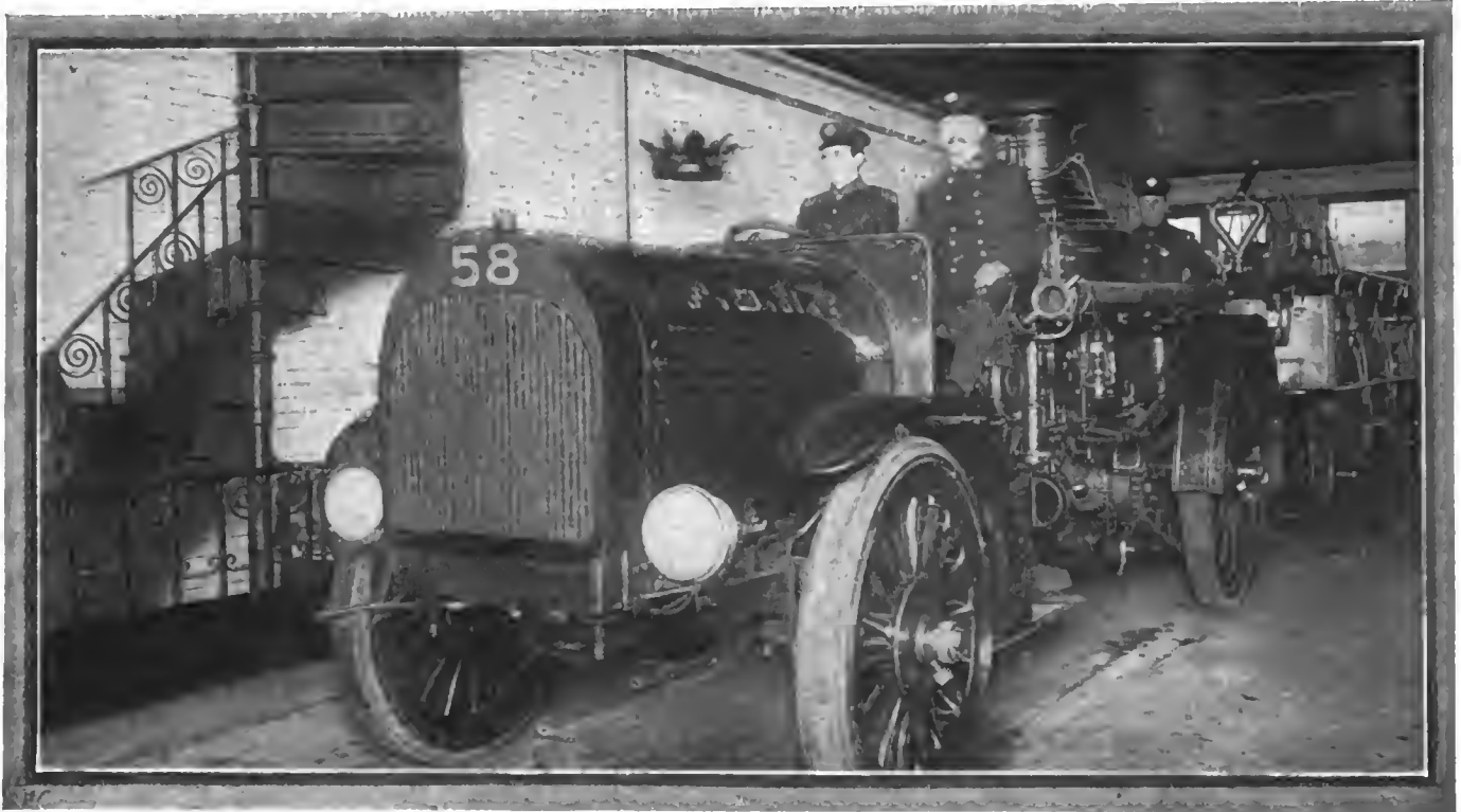
110-horsepower Notl tractor ready to pull its pumping engine to the fire
